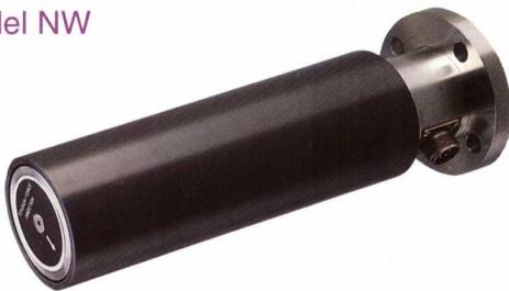
Specially designed for narrow webs in single-side frame machines. Combines an idler roll and two tension transducers in one unit—for fast, easy installation and high accuracy. Three widths accommodate narrow webs up to 14" (356mm) wide. Load ratings of 12 lbs. (55N) to 100 lbs. (450N) Choose a single-bolt mounting or four-bolt flange.
