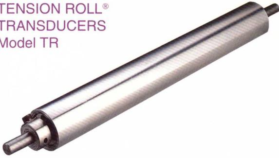
Tension transducers and dead-shaft idler roll are combined in one integral unit. No assembly is required. Faster, easier, and cheaper to install than separate roll and transducers. Only one transducer cable—eliminates cable crossing between machine frames. Various roll diameters are available, starting at 4"(100mm). Available in face widths of 7"(177mm) to over 120"(3048mm).
